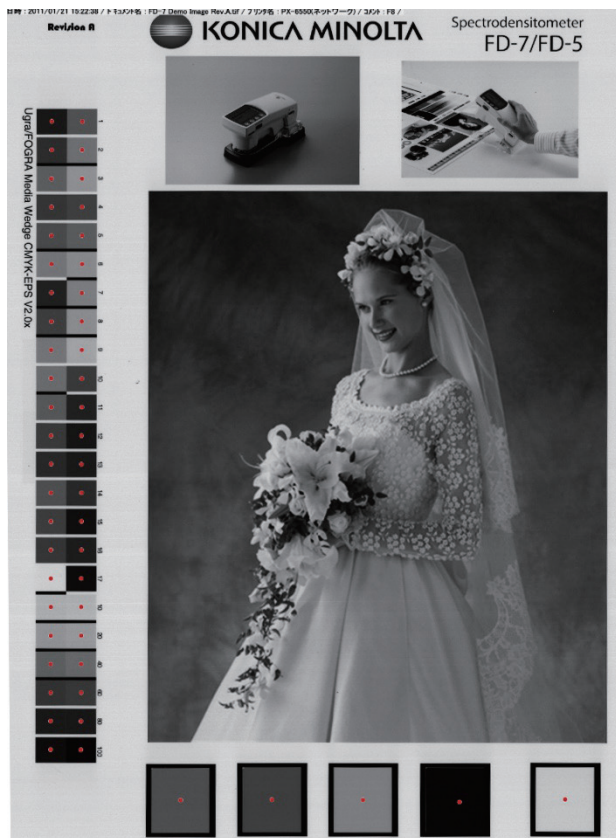
Fig. 9 The automatic location of measurement points. Red points indicate the located centers of the patches.
